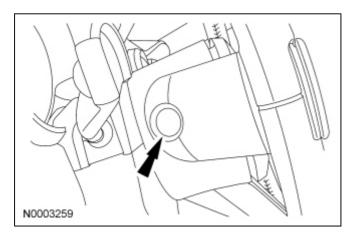
8. Remove the 2 driver air bag module bolts (1 shown).
