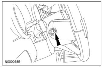
13. Install the 2 driver air bag module bolt caps (1 shown) in the steering wheel.
