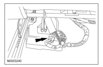
5. Remove the Restraint System Diagnostic Tool from the vehicle harness side of the passenger side air bag module electrical connector.
