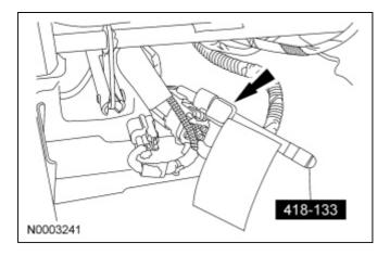
4. Connect the driver side air bag module electrical connector and reset the red locking tab.
