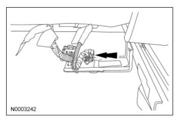
7. Remove the Restraint System Diagnostic Tool from the vehicle harness side of the passenger air bag module electrical connector.
