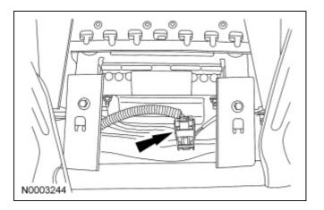
13. Attach the Restraint System Diagnostic Tool to the vehicle harness side of the passenger air bag module electrical connector.
