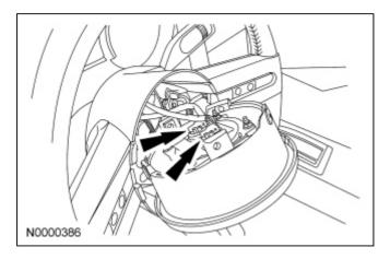
10. Attach the Restraint System Diagnostic Tool to the clockspring electrical connectors.
