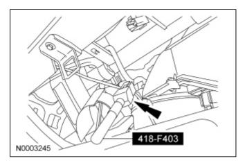
8. Connect the passenger air bag module electrical connector.
