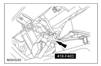
14. Release the red locking tab and disconnect the passenger side air bag module electrical connector.
