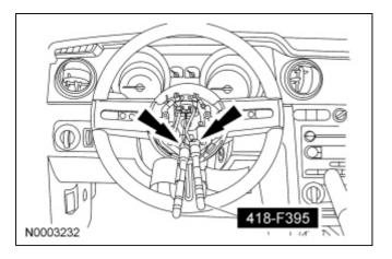
11. Connect the 2 electrical connectors and position the driver air bag module.
