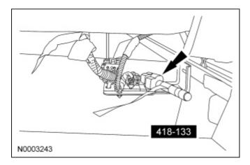
6. Connect the passenger side air bag module electrical connector and reset the red locking tab.
