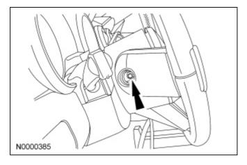
9. Disconnect the 2 electrical connectors and remove the driver air bag module.
