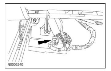
17. Attach the Restraint System Diagnostic Tool to the vehicle harness side of the driver side air bag module electrical connector.
