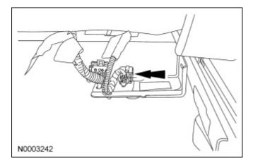
15. Attach the Restraint System Diagnostic Tool to the vehicle harness side of the passenger side air bag module electrical connector.
