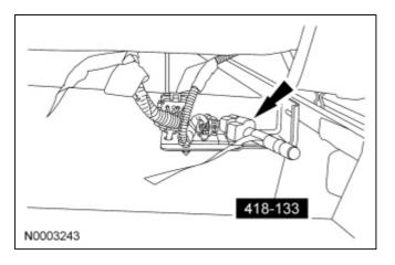
16. Release the red locking tab and disconnect the driver side air bag module electrical connector.
